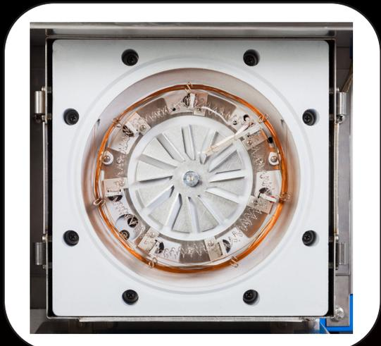
Low sensitivity analysis (ppm to ppb) is achieved by combining the precision and responsiveness of the Eclipse ovens, state-of-the-art programmable electronic pressure and flow controls, and the most sensitive GC detectors on the market.
